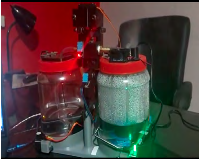
Figure 14. Fuzzy Logic Type-2 is used to determine times of humification in a room analyzed the ambient temperature.
