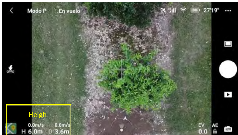
Figure 1: Application interface that shows the height of the drone.
